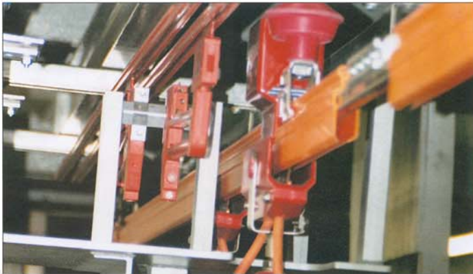
A solid-steel frame, aluminum enclosure, convex spring-loaded collector shoes and permanently sealed wheels assure effortless operation.
